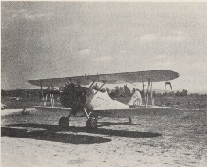
FIG. 2. N3N AIR TANKER, 200 GALLONS CAPACITY. THREE OF THESE AIRCRAFT WERE USED IN THE INITIAL ATTACK EXPERIMENT.
